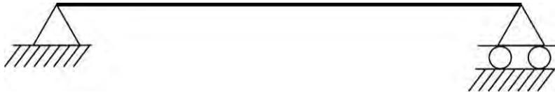
**Figure 21** Simple-span beam with statically determinate boundary conditions.
